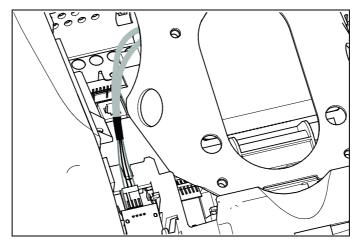
Figure 14: Connecting the heart rate cable
